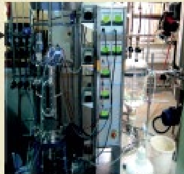
Proto scale fermentative production of H_2 from xylose in 30 liter scale bioreactor (no working volume)
