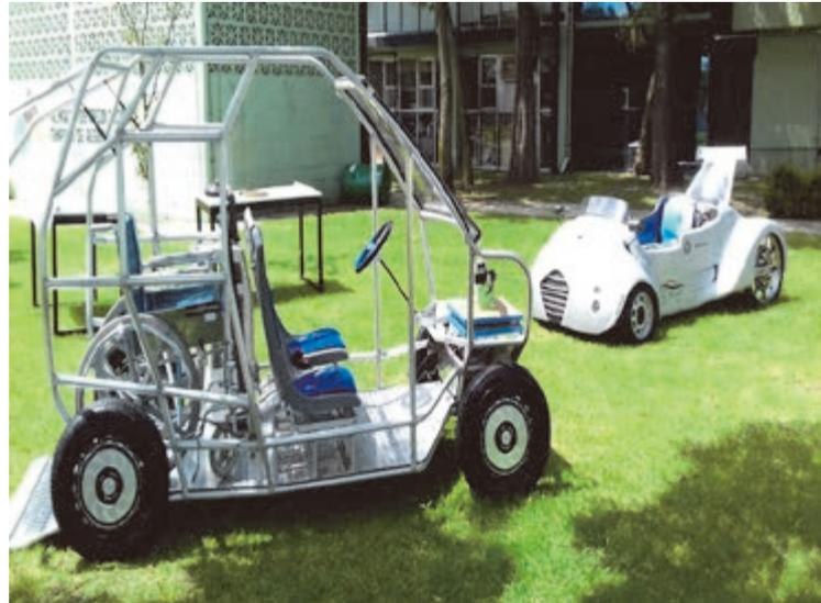
Prototype Vehicles propelled by fuel cells built in Cinvestav-Mexico City
