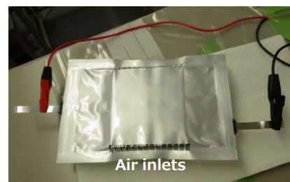
Fig. 3. 10-cell module with Li-air batteries stacked in parallel.
